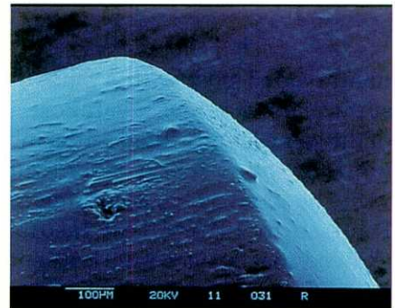
Figure 11—The Compositest™ surface treated with ALL-BOND® 2 Adhesive System Primer B. The surface is very smooth, fully covered, and impregnated by a thin primer layer that is impossible to divide from the resinous matrix of the Compositest™ (SEM, X150).
