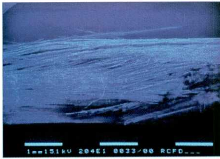
3. Sample of Group 6 after the fracture following the fatigue test. The separation between the fibers and the resin matrix is evident.
