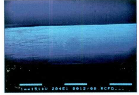
5. Sample of Group 4. After 2,000,000 cycles the post is still intact. The point at which the load was applied is evident, with a small depression in the middle of the post, which in any case remains perfectly intact from a structural point of view.
