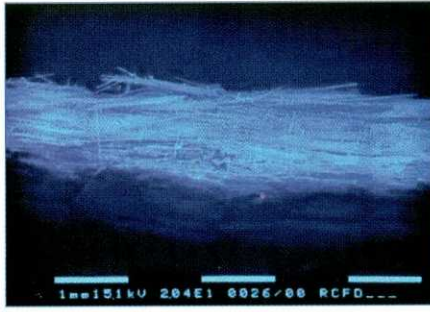
4. Sample of Group 2. Here too the fracture shows the failure of the bond between the fibers and the resin matrix.
