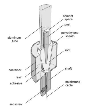
Fig. 2 – Schematics of the specimens. The root was sheathed into a polyethylene hose and encased into resin (i.e. the bone analog). The resin was housed in a container featuring a shaft to be griped into a rotating collet. The root was prevented from escaping its resin housing by a multistrand cable that was crew-fastened to the shaft. An aluminum tube that was cemented onto the post's head served as crown analog.
