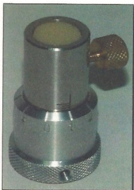
Fig. 1. The custom made cylindrical mold used for specimen fabrication.
